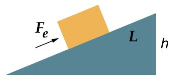
An inclined plane is a device such as a ramp, stair, or ladder and is used to more easily raise a load. The steepness of the incline affects the level of ease of movement. While a shallow incline makes it easier to raise a load, the length of the incline must be longer to compensate.
