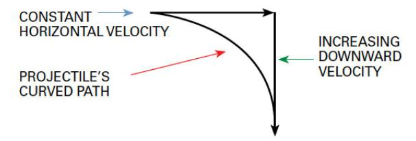
(d) The difference between forward velocity and acceleration due to gravity.
